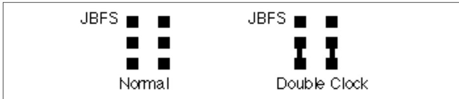
Proper operation from either the on-board oscillator or the cascade clock input requires that JBFS be set in the normal mode.
