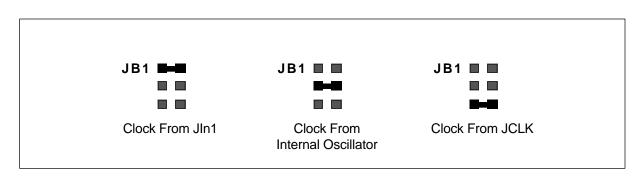
Use the silk screened label "JB1" as a reference for determining the correct jumper position.
